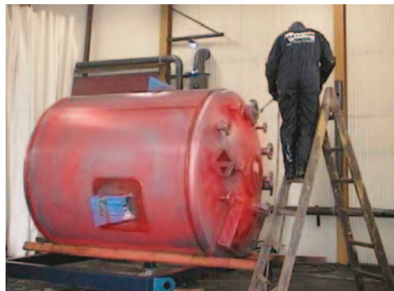
Avesta RedOne™ Pickling Spray 240 – spray pickling with Best Available Technique.
