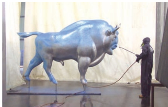
Avesta BlueOne™ Pickling Spray 230 – spray pickling with Best Available Technique.
