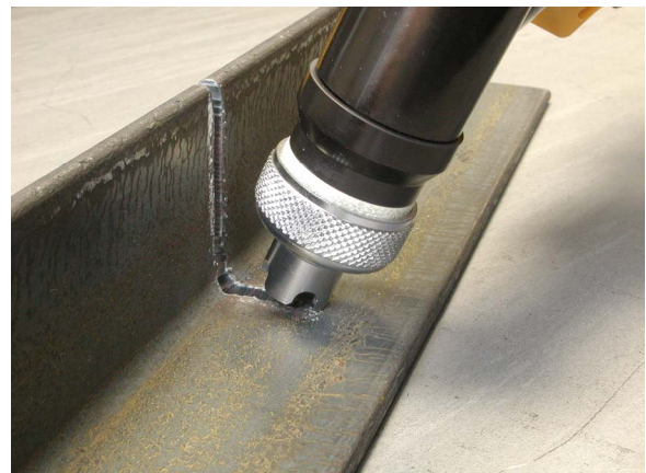
Fig. 16: Cutting with long consumables
